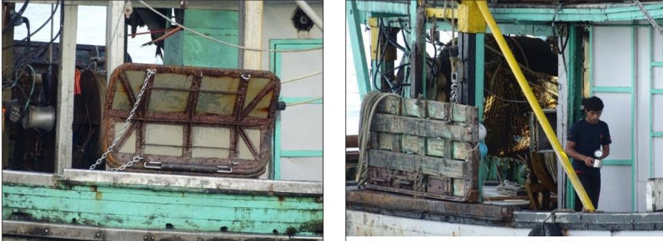
Figure 1: Otter Trawl (rectangular board) onboard fish trawlers in Sabah.
