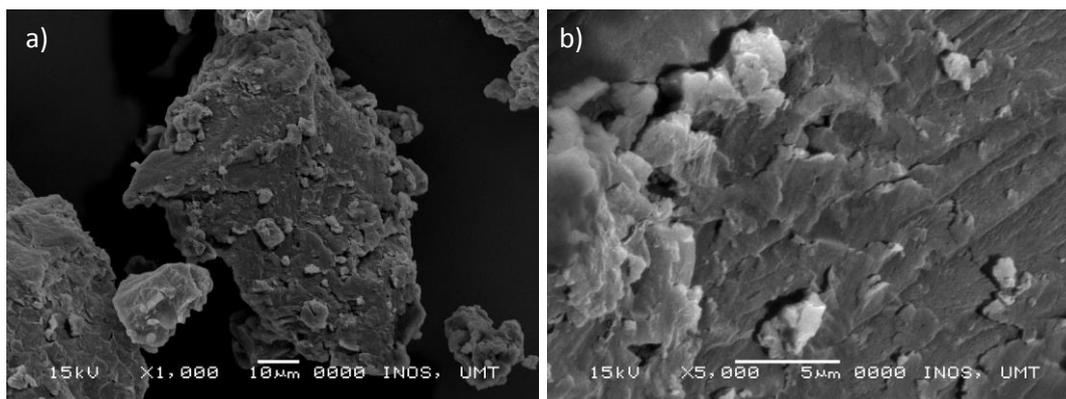
Figure 5: SEM micrographs of NiAL at magnifications of a) 1000X b) 5000X
