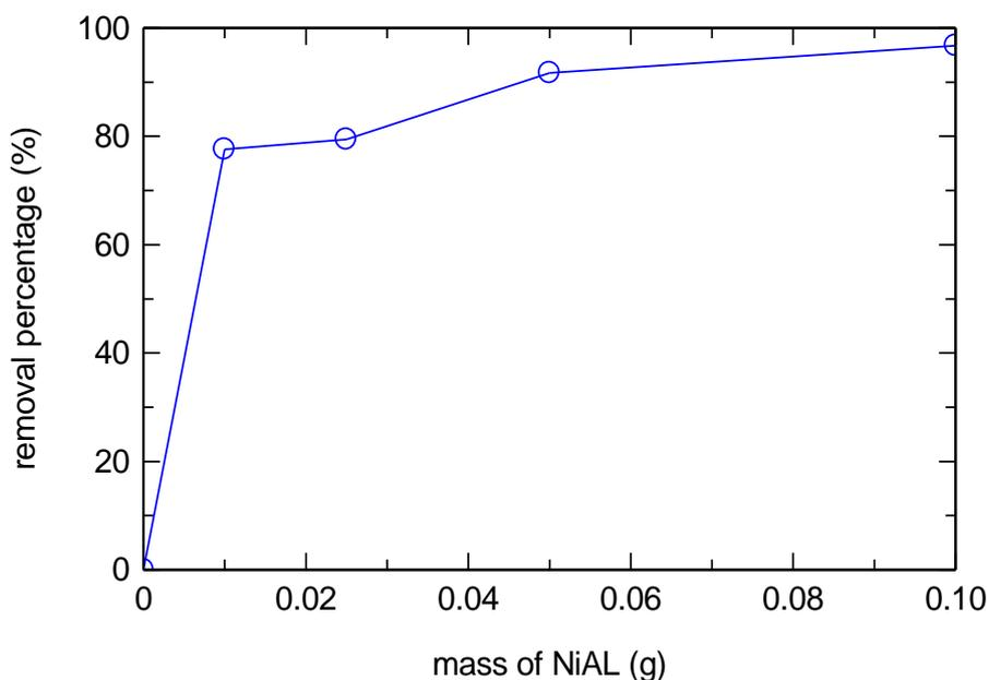
Figure 6: Removal percentage of EBT at different masses of NiAL
